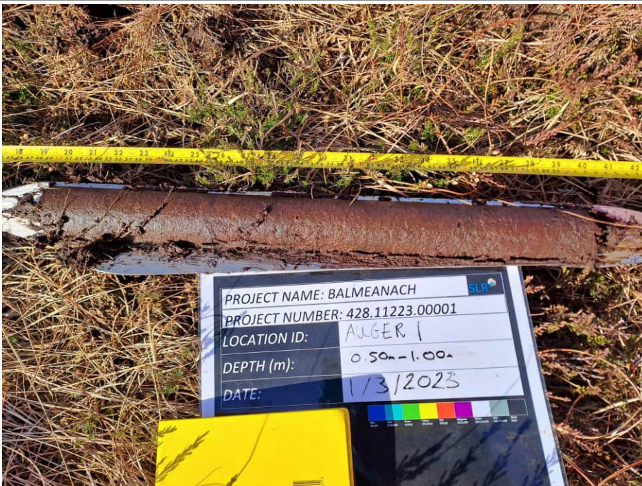
Photograph 2: Auger 1 (0.50m – 1.00m)
