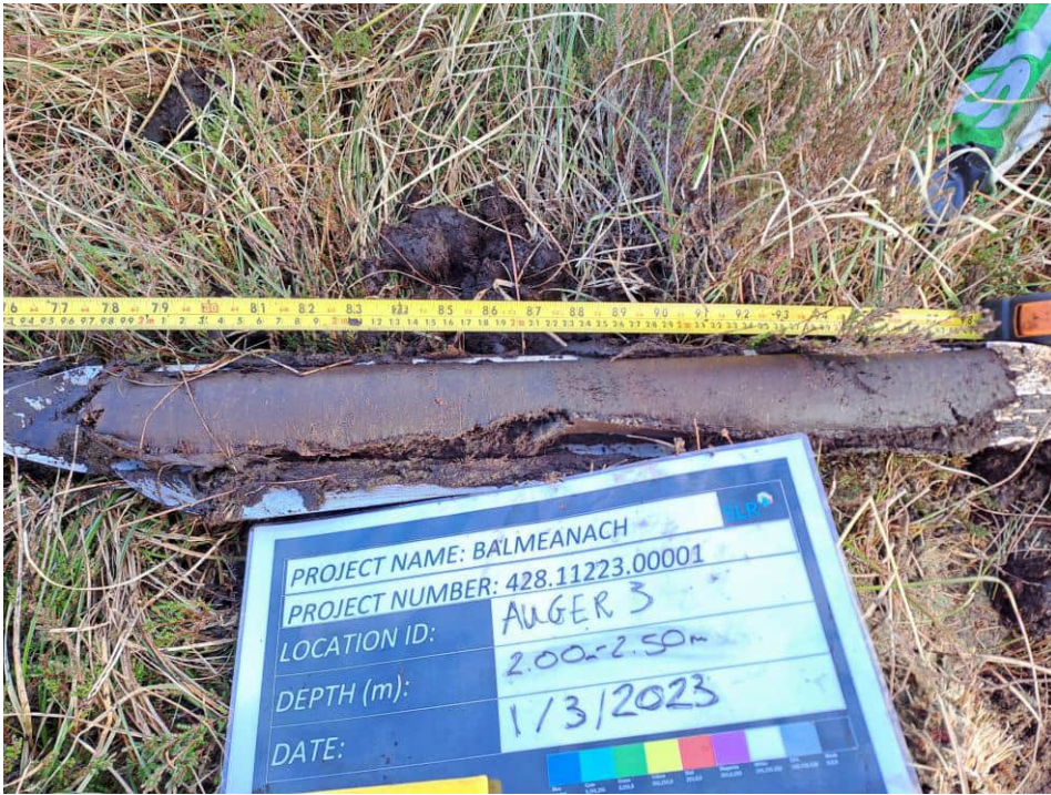
Photograph 15: Auger 3 (2.00m – 2.50m)
