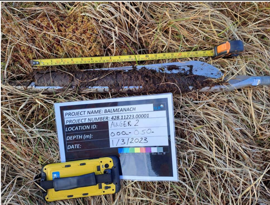
Photograph 6: Auger 2 (0.00m – 0.50m)
