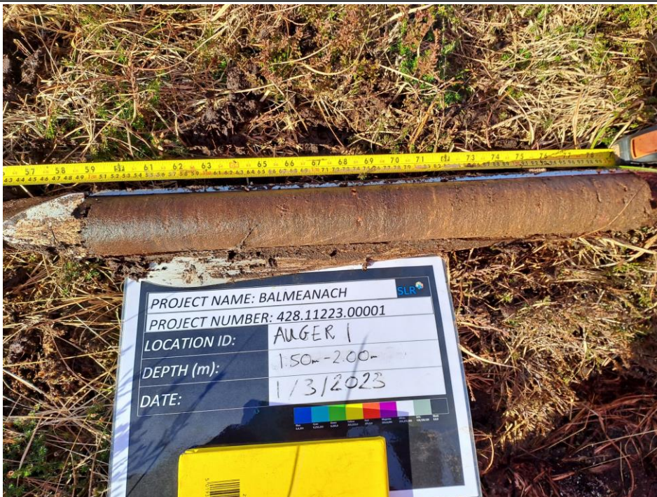
Photograph 4: Auger 1 (1.50m – 2.00m)
