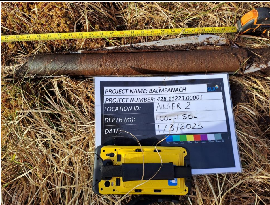
Photograph 8: Auger 2 (1.00m – 1.50m)
