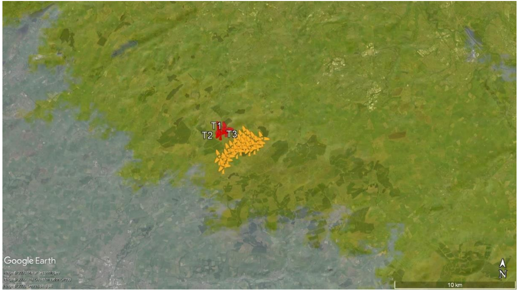
Figure 10: Visual LoS coverage at 149.9 metres AGL from Cumbernauld
