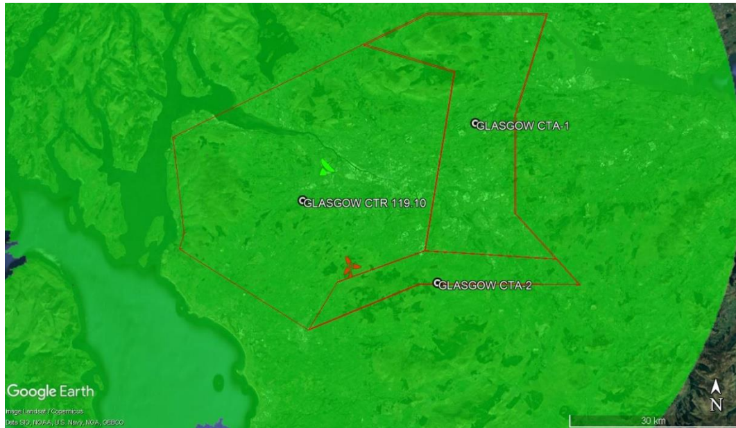
Figure 24: Visual LoS Coverage of the airspace above the proposed wind farm by the Glasgow airport radar at 5000 feet ASL
