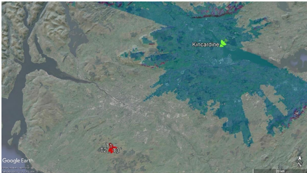
Figure 13: Visual LoS coverage at 149.9 metres AGL from Kincardine radar
